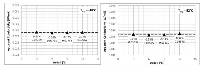
The polyiso insulation data were first analyzed using the TCI method, assuming an equation with cubic form. The presentation elaborates on this process. Analysis of data from the deltaT=28°C tests results in a different temperature-dependence curve than that produced by analysis of the deltaT=12°C tests. Neither of the TCI curves adequately predicts the results for the small deltaT tests.
