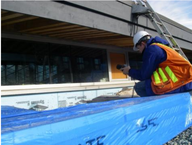
Fig.5.9 Typical Infrared Camera Used for Air leakage Diagnostic Testing
