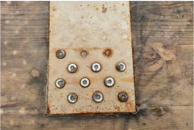
g) Failure of structural fasteners caused by swelling of the wood and corrosion on fasteners.
