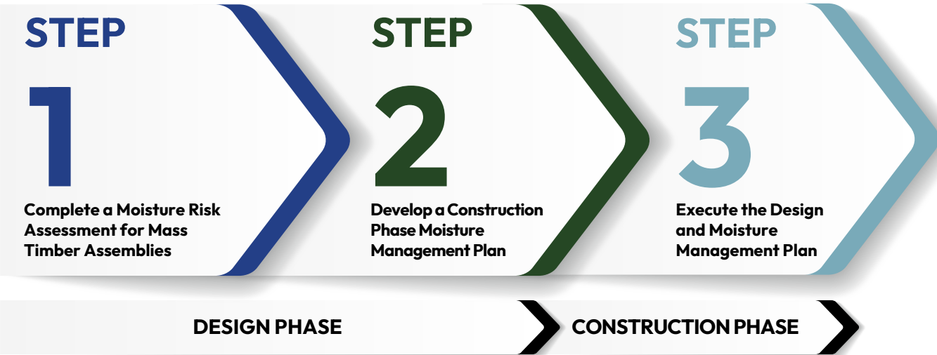
Figure 4 The three-step moisture management process relative to the project phase.
