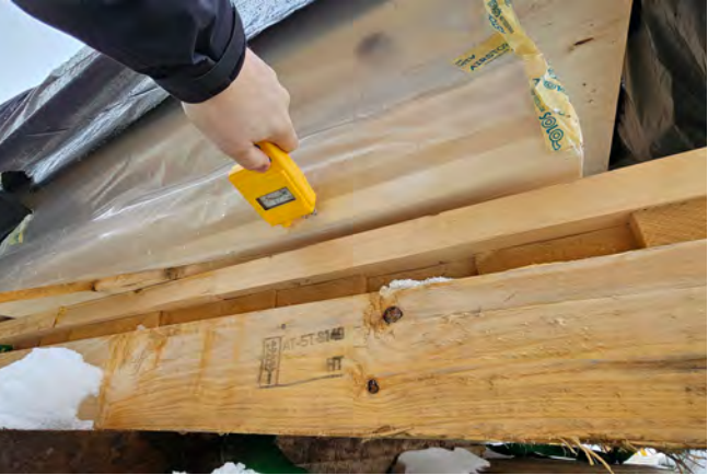
Figure 65 A worker takes a moisture content reading of a CLT panel that is stored on-site as part of the regular monitoring requirements outlined in the project's moisture management written plan.
