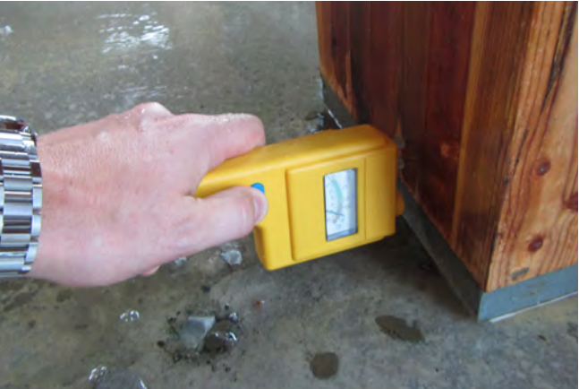
Figure 64 Moisture content reading taken at the base of a mass timber column that has been exposed to moisture.
