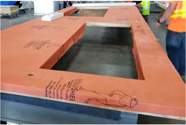
Figure 26 CLT wall panels with factory-installed air barrier and WRB membrane and window rough opening membranes prior to on-site installation of windows and panel joints.
